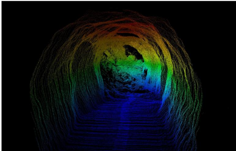
FIGURE 2. Record from scanning of collapsed area by ROV.
