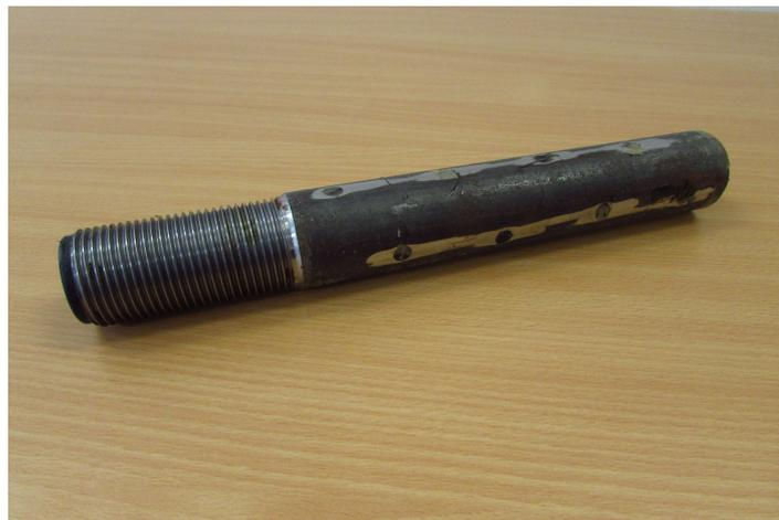
FIGURE 5. Anchor for a cyclic test of bare bars.
