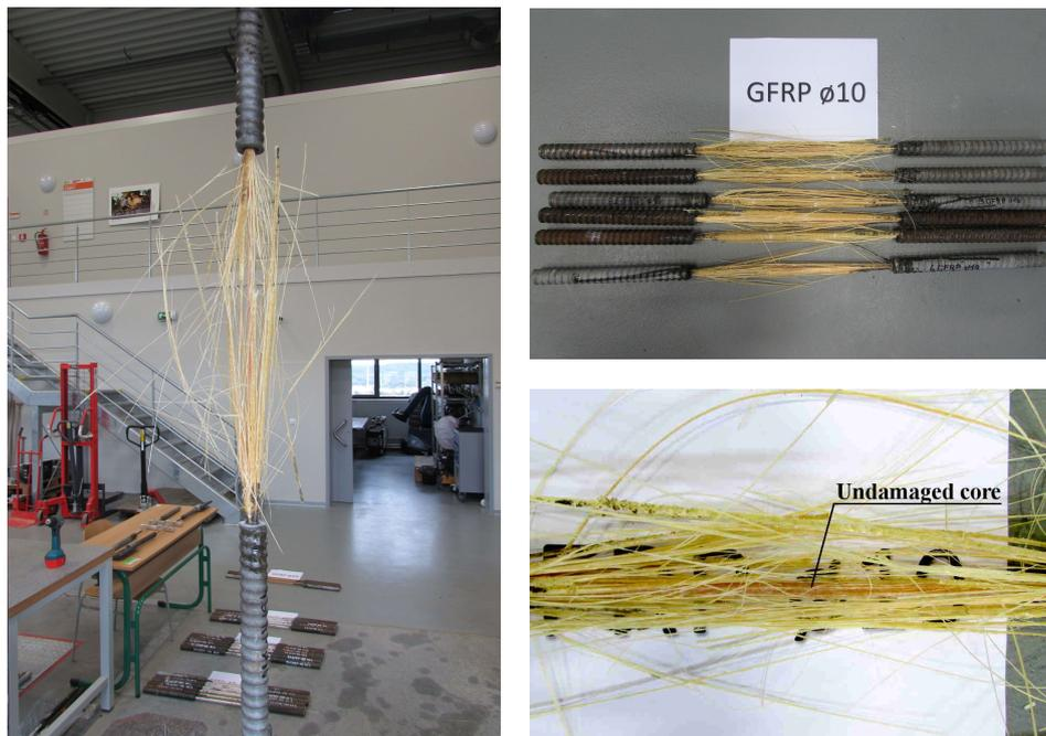
FIGURE 1. Failure of samples during monotonic test.
