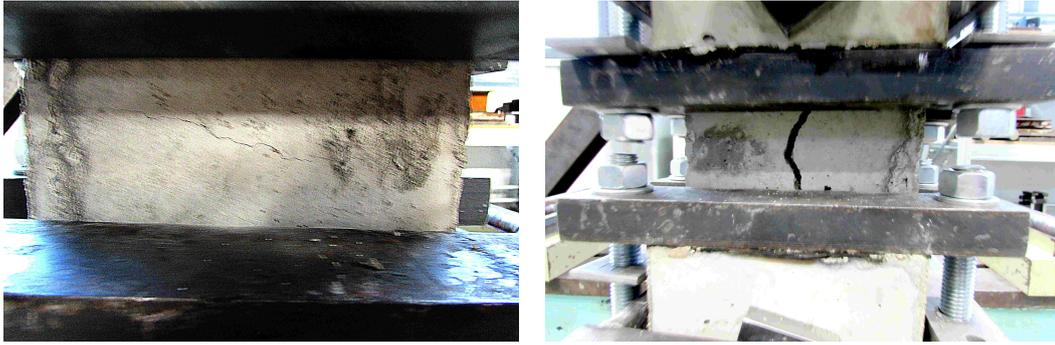
FIGURE 8. Transverse (left) and longitudinal (right) crack during cyclic loading.
