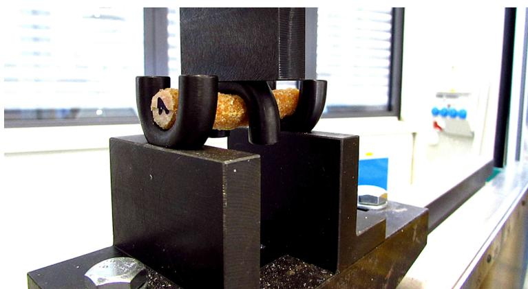
FIGURE 3. Configuration of interlaminar (longitudinal) shear test.
