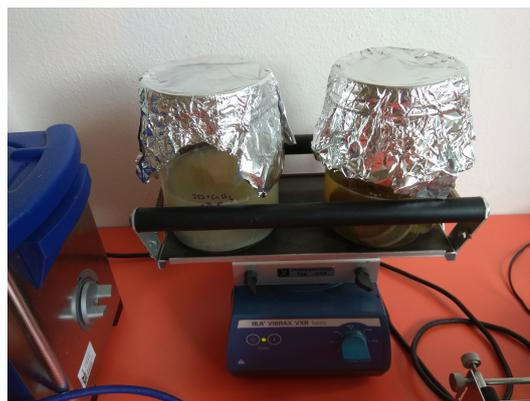
FIGURE 4. Concrete specimens in media (253 media on the left, 253 media with 2% CaCl<sub>2</sub> solution on the right).
