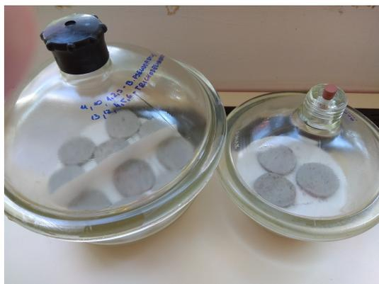
FIGURE 6. Concrete specimens in desiccators.
