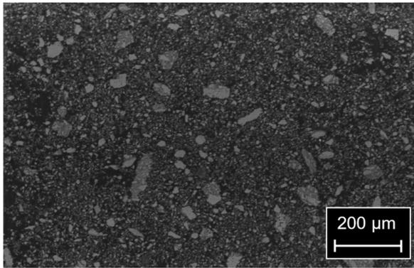
FIGURE 1. The image of micronized marble powder, magnified 100 $\times$ , BSE detector.
