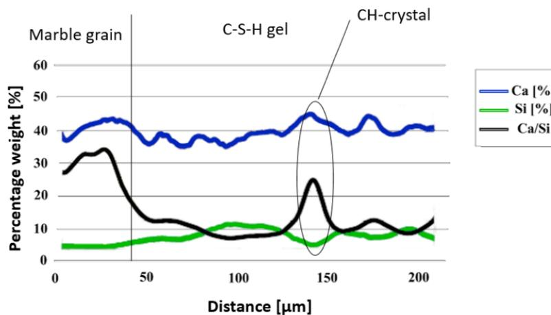
FIGURE 4. Concentration of calcium and silicon in line scan.
