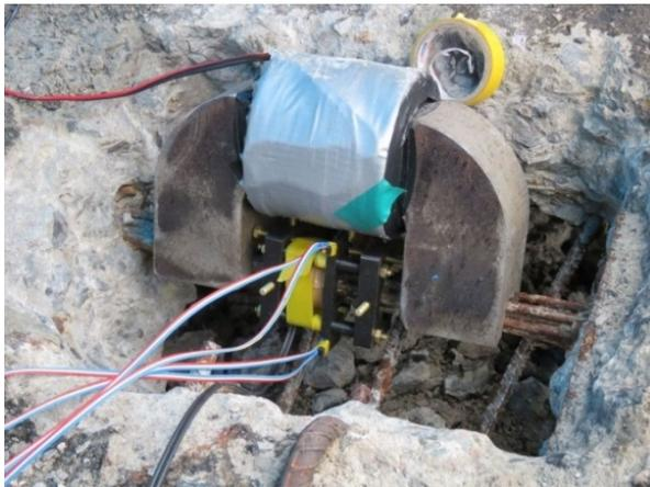
FIGURE 4. The complete EM sensor on the cable.
