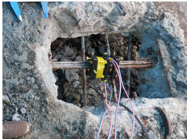
FIGURE 3. The holder for the set of four Hall sensors with the embedded secondary coil 1 positioned on the studied cable.
