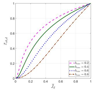
FIGURE 7. The influence of different levels of ambient relative humidity on the drying creep vs. drying shrinkage kinetics according to the B3 model. The remaining parameters are from the first line in Tab. 1.
