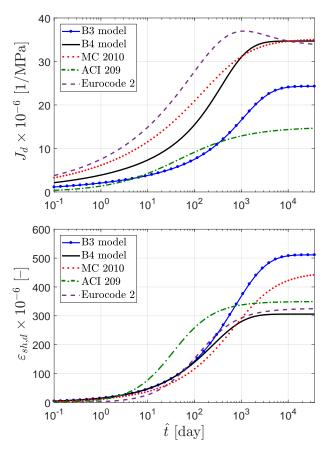
FIGURE 1. Drying creep compliance curves (top) and drying shrinkage curves (bottom) given by the analyzed design codes and prediction models.
