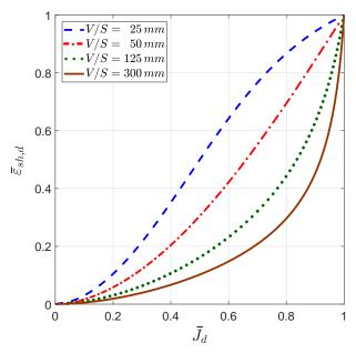
FIGURE 8. The influence of different V/S ratios on the drying creep vs. drying shrinkage kinetics according to the *fib* MC 2010 model. The remaining parameters are from the first line in Tab. 1
