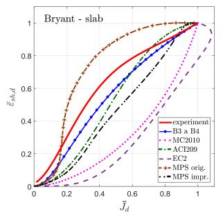
FIGURE 9. The comparison of the experimental data, prediction models and FE simulations of the Bryant's experiment, 2V/S = 150 mm (slab).
