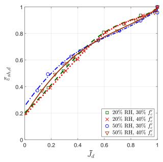
FIGURE 5. Comparison of normalized drying shrinkage and normalized drying creep evaluated from the experiments of Keeton at 20 % and 50 % relative humidity and two levels of loading.  $f'_c$  is the compressive strength at the age of loading. Points are the experimental data.
