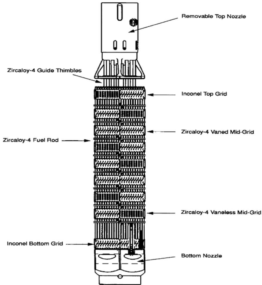
FIGURE 1. VVANTAGE-6 fuel assembly [11].
