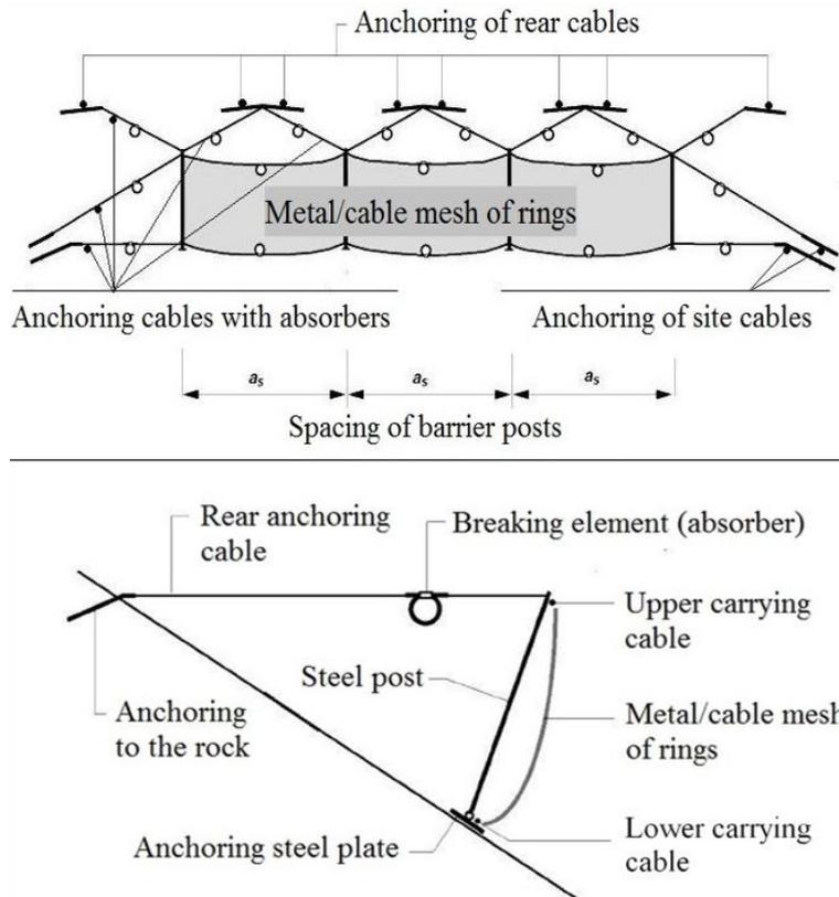
FIGURE 6. Dynamic barrier – schematic view and cross section.
