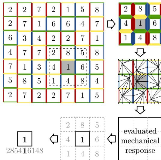
FIGURE 9. Local tiling process: macro tiling  $\Rightarrow$  local tiling  $\Rightarrow$  local FE mesh  $\Rightarrow$  evaluation  $\Rightarrow$  cropping results  $\Rightarrow$  results for tile  $T_i$ .
