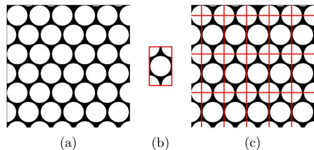
FIGURE 2. Modelling of periodic microstructure, a) periodic microstructure, b) PUC, c) reconstructed microstructure.
