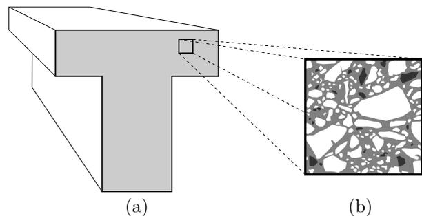
FIGURE 1. The appearance of the structure at different scales, a) homogeneous at macro-scale, b) heterogeneous at micro-scale.
