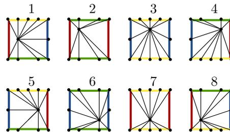
FIGURE 8. Mutually edge-compatible finite element meshes on tiles.
