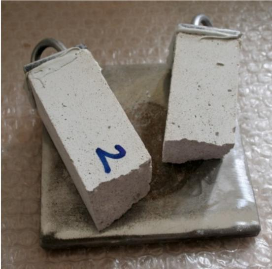
FIGURE 9. Failure of specimen M2.
