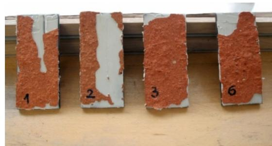
FIGURE 4. Failure of specimens no. 1, 2, 3 and 6.
