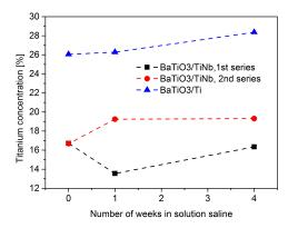
FIGURE 3. Titanium concentration due to an action of solution saline.
