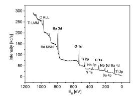
FIGURE 1. Photoelectron spectrum  $BaTiO_3$  on TiNb substrate after preparation of sample. Visible peaks (photoelectron as well as Auger) are marked, those used to calculation of element concentration are in bold.
