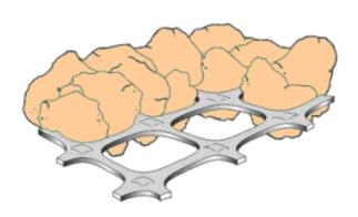
FIGURE 2. Reinforced geogrid Tensar SS.
