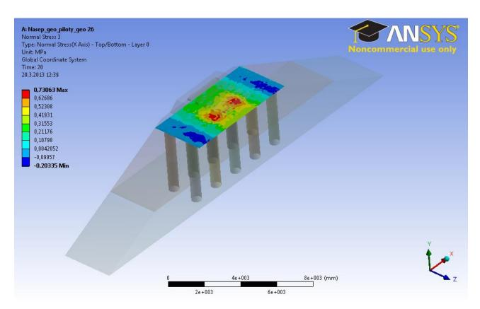
FIGURE 13. Stress field  $\sigma_x$  of the geogrid of the embankment reinforced by the geogrid and the columns sheathed a geogrid.
