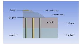
FIGURE 5. The scheme of layers in the model of reinforced earthworks.
