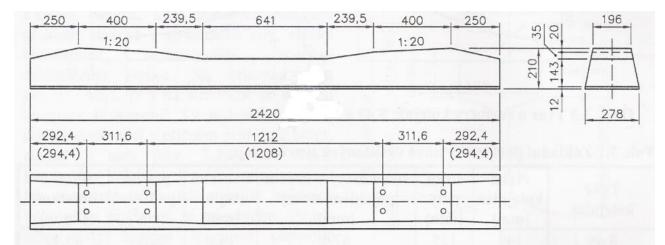
FIGURE 7. The concrete sleeper [mm].
