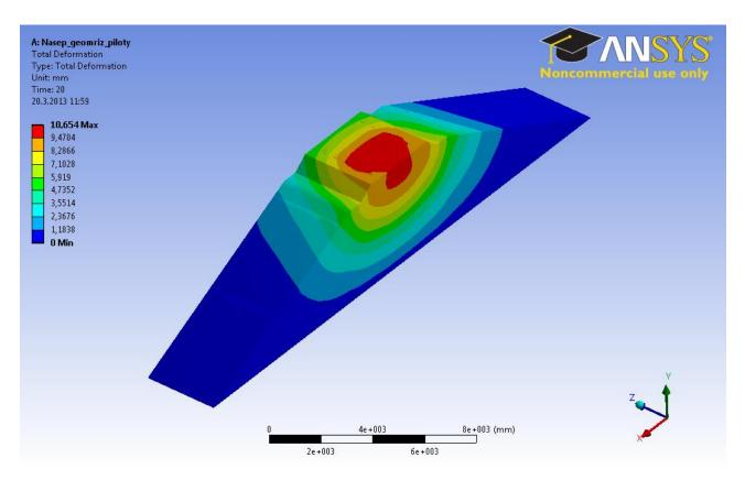
FIGURE 11. Total deformation of the embankment reinforced by the geogrid and the columns.
