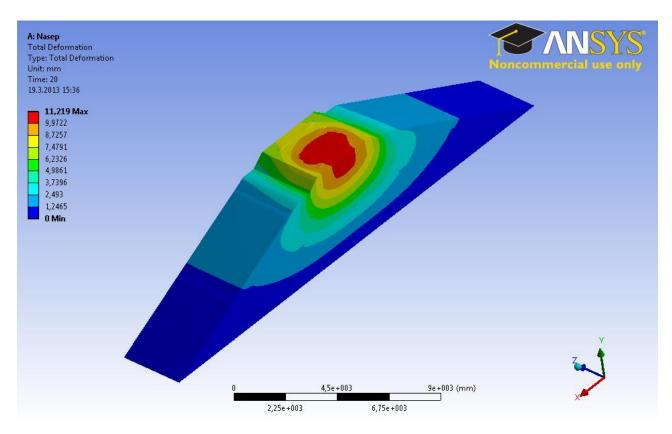
FIGURE 9. Total deformation of the non-reinforced embankment.
