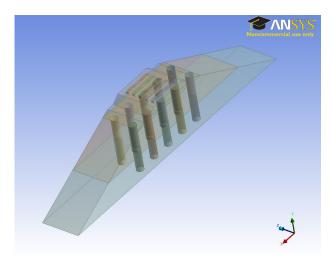
FIGURE 6. The model of the embankment with a geogrid and lime-cement columns.
