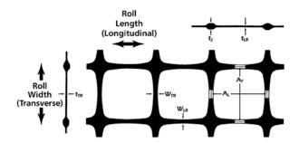
FIGURE 8. Shape and sizes of geogrid TENSAR SS30.
