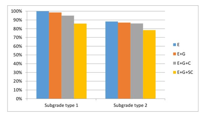
FIGURE 14. Total deformation of the embankment for all four types of structure and for two types of subgrade with various modulus of elasticity.
