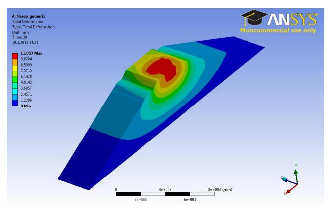
FIGURE 10. Total deformation of the embankment reinforced by the geogrid.
