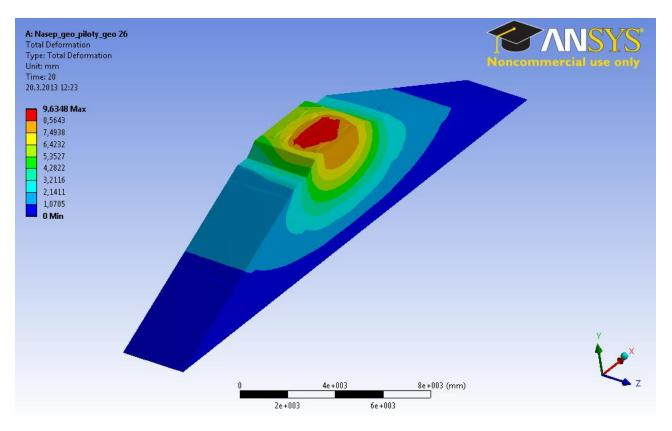
FIGURE 12. Total deformation of the embankment with the geogrid and the columns sheathed a geogrid.
