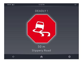
FIGURE 1. One-stage warning GUI.
