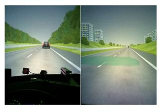
FIGURE 5. Highway simulation with dangerous events.
