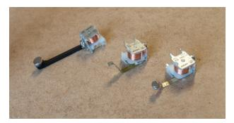
FIGURE 9. Examples of three types of control sections (from left to right): parking space, stop section and branch-off junction – an alternative to Faller elements.
