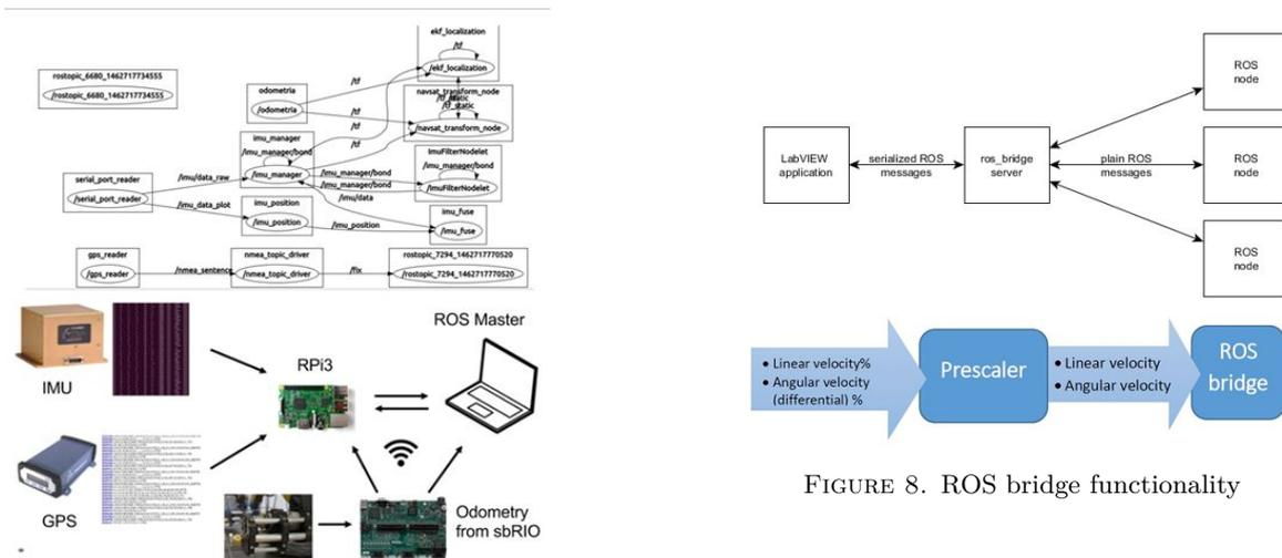
FIGURE 7. Raptors rover navigation system (up) nodes and topics of the ROS structure (down)
