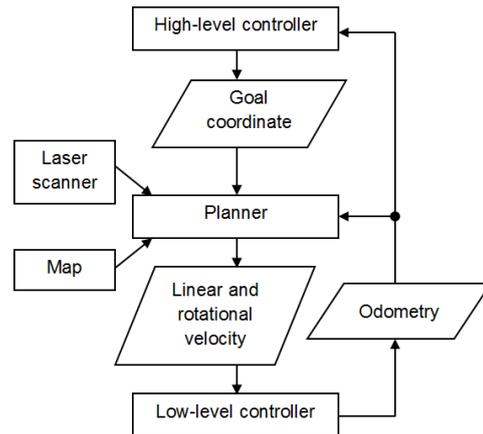
FIGURE 2. Control system of the HusarX robot
