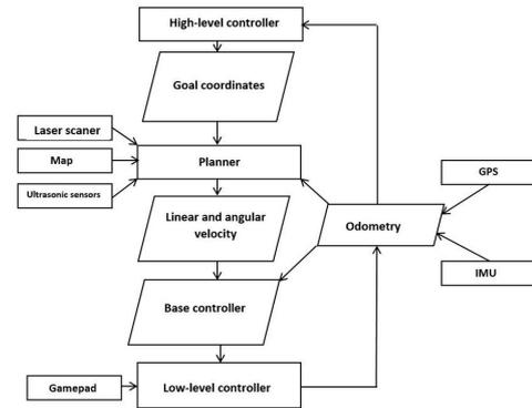
FIGURE 11. Navigation structure of the Quadron robot
