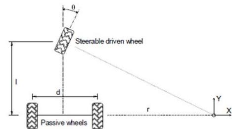
FIGURE 12. Kinematics of the Quadron robot
