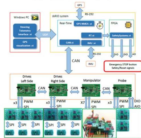
FIGURE 6. The Raptors rover and its control system
