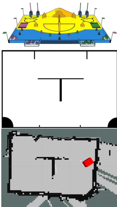
FIGURE 4. Building the navigation map (middle) based on the geometry of playing board (up) of Eu-robot competitions, or based on several scans taken on the real board (down)
