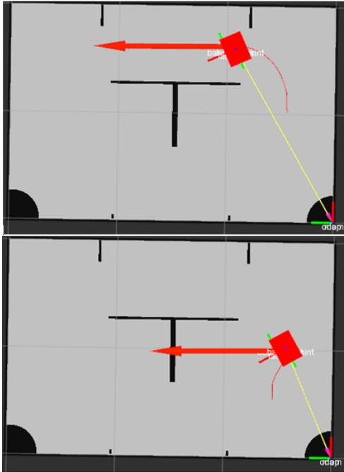
FIGURE 5. Rviz screens presenting two consecutive steps of planning robot's movements (red line), red arrow shows orientation of the robot required in the step
