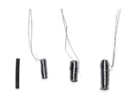
Fig. 6: Examples of bare coils made of self-bonding copper wire and a ferromagnetic core 8 mm in length. From the right 2000 turn coil, 1000 turn coil and 500 turn coil.
