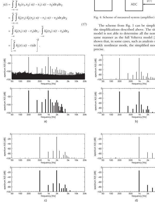
Fig. 5: Comparison of responses to a) 200 Hz and 1 kHz tones, up to -150 dB; b) 200 Hz and 1 kHz tones, up to -100 dB; c) 500 Hz and 2 kHz tones, up to -100 dB; d) 1 kHz and 5 kHz tones, up to -100 dB; SONY SDP-300 - above, model - below
