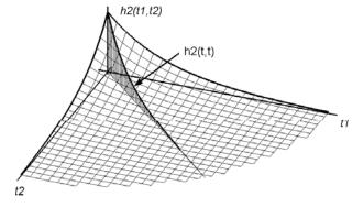
Fig. 2: Example of second-order Volterra kernel
