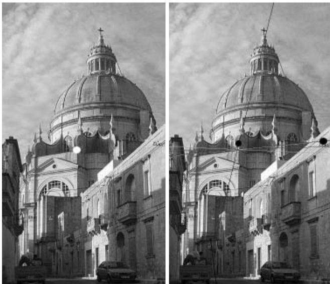
Fig. 3: Example of an image pair with points and their respective line with minimal k^2 : We see the estimated epipolar line in the second image, \mathbf{l} , that corresponds to the point \mathbf{x} in the first image, which is marked by a white point. The epipolar band for a value k^2 = 5.9915 , respectively a probability \alpha = 0.95 is within the hyperbola. Points marked by a black circle in the second image are shown together with the lines of minimal k^2 , denoted by \mathbf{m} , and represented dark.
