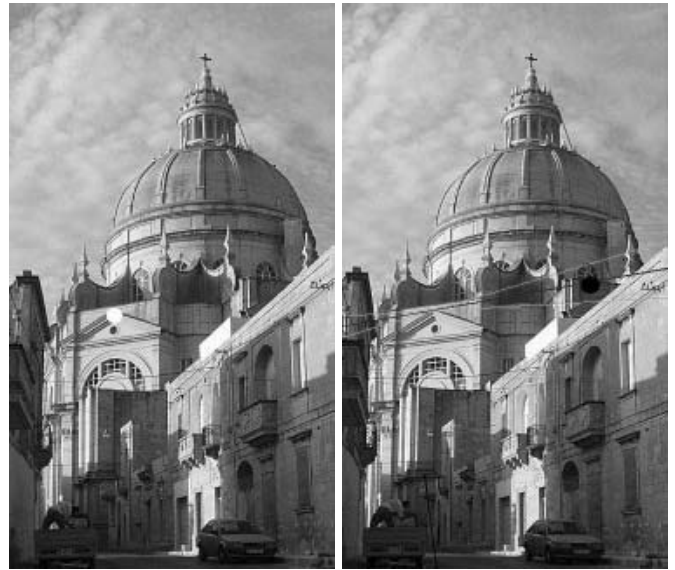
Fig. 4: Line with minimal k^2 computed for a point on the estimated epipolar line: We see the epipolar band for a value k^2 = 5.9915 , marked by the hyperbola, corresponding to the point \mathbf{x} in the first image, which is marked by a white point. Obviously the epipolar line with smallest k^2 for points on the estimated epipolar line is the epipolar line itself. Here we see that these two lines are superposed. The corresponding value is k^2 = 0 .
