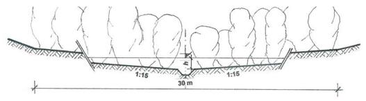
Fig. 10: Cross section of the proposed natural channel and its surroundings
