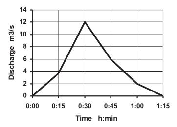
Fig. 8: Deduced hydrograph in the existing channel above Rozhovice during the flood event on May  $30^{\rm th}$ , 2005
