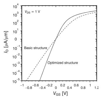
Fig. 11: Transfer characteristics of the basic and the optimized structure
