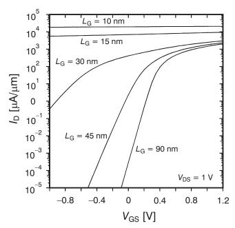
Fig. 5: Transfer characteristics at different gate lengths
