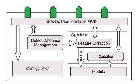
Figure 7: Software architecture
