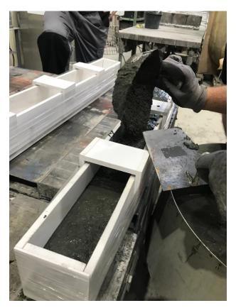
FIGURE 1. The filling of moulds.
