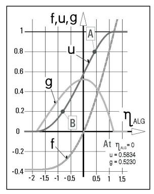
Fig. 17: Complete solution of the planar mixing layer profiles – of relative velocity u, its gradient g, and the relative stream function f – using the algebraic model of turbulence. Eq. (42) integrated using the Runge-Kutta algorithm and the indicated boundary condition values at  $\eta_{ALG} = 0$ .
