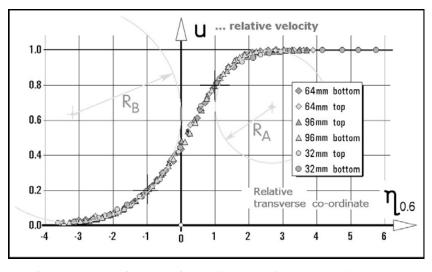
Fig. 13: Velocity data evaluated from Fig. 12 and re-plotted in similarity variables. No significant effect of transversal curvature (which increases with  $X_1^*$ ) was found. The different osculation radii  $R_A$  and  $R_B$  indicate lack of central symmetry, a feature of the usually presented Görtler's solution in its first-term form Eq.(4).
