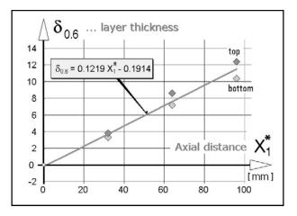
Fig. 14: Convention thickness  $\delta_{0.6}$  dependence on the downstream distance  $X_1^*$ . Resultant least-squares expression is fitted through all experimental data as a mean between the not perfectly symmetric top and bottom sides of the jet.
