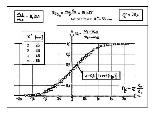
Fig. 8: Velocity profiles of the mixing layer, Figs. 3 and 4, plotted in the similarity co-ordinates and compared with the first-term Görtler solution Eq. (4). No significant systematic effect of the transverse curvature is discernible.
