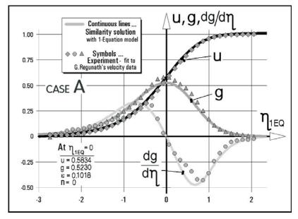
Fig. 21: Initial attempt at a solution using 1-equation model compared with the experiment. Profiles computed from the starting conditions at  $\eta_{1EQ} = 0$  with the solution parameter  $c_z/(ks)$  exactly as used earlier with the algebraic model for equilibrium turbulence – Eq. (47).
