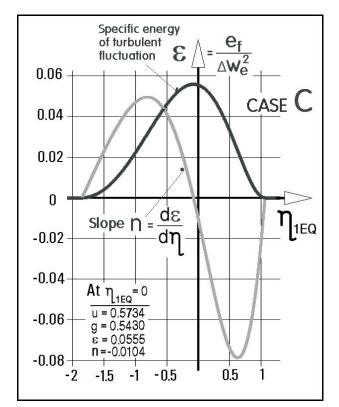
Fig. 22: Similarity transformed fluctuation energy profiles in the mixing layer obtained with the 1-equation model solution using the conditions at  $\eta_{1EQ} = 0$  adjusted so that the integration proceeded to the ideal zero value boundary conditions on both sides of the layer
