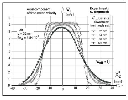
Fig. 12: Velocity profiles obtained by PIV measurements in an air jet (data obtained in collaboration with G. Regunath). Only three profiles nearest to the exit were used for the comparison with the similarity solutions. The slight asymmetry of the profiles is hardly avoidable in practical flows.
