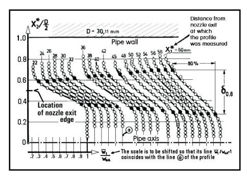
Fig. 5: Unpublished 1978 measurements by a miniature Pitot probe of axial time-mean velocity profiles in the mixing layer inside the pipe of Fig. 3. Convention thickness  $\delta_{0.8}$  is defined as the distance between the black symbols, where the velocity differs by 10 % from the velocity outside the layer.
