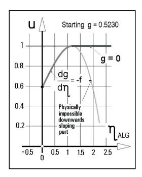
Fig. 16: With g = 0.523 the solution curve just reaches u = 1 at the vertex of the parabola. Thereafter, the physically unacceptable decrease is avoided by switching from the solved equation  $dg/d\eta = -f$  to the other alternative g = 0.
