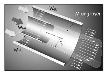
Fig. 2: A transversally curved mixing layer forms when flow of higher velocity  $w_{eA}$  leaves the central nozzle and mixes with the outer flow of lower velocity  $w_{eB}$ . Transversal curvature radius varies with axial distance differently than the layer thickness. This renders an exact similarity of the profiles impossible.
