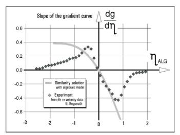
Fig. 20: Comparison of the profiles of  $dg/d\eta = d^2 u/d\eta^2$  obtained by the similarity solution and by the experiment. According to the primary alternative of Eq. (42), the values are also negative values of the transformed stream function *f*.
