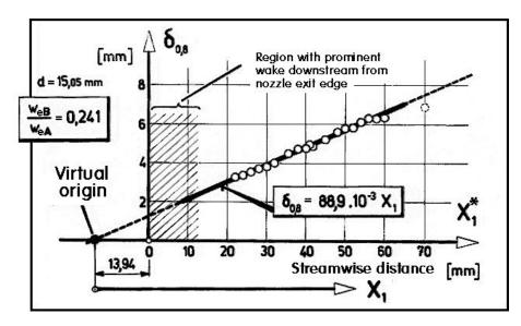
Fig. 6: Streamwise dependence of the convention thickness  $\delta_{0.8}$
