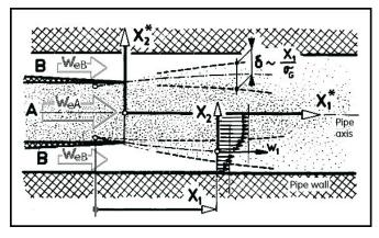
Fig. 4: The mixing layer in a round pipe: faster flow A injected into parallel flow B of lower velocity  $w_{eB}$ . Investigations of this layer were performed by the present author in 1978 at CTU in Prague as a part of classified study of radioactive contaminant diffusion towards the pipe wall.
