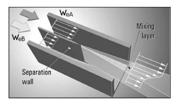
Fig. 1: Mixing layer between parallel flows is quite thin because momentum diffusion from the flow of higher velocity  $w_{eA}$  towards the lower velocity  $w_{eB}$  is slower than the streamwise motion. The character of the flow is here represented by time-mean velocity profile.
