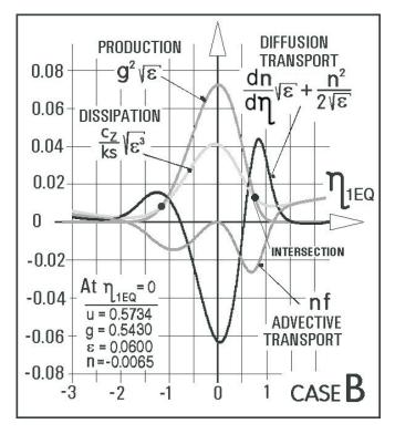
Fig. 24: Another 1-equation model solution, computed for a slightly increased starting value of fluctuation energy  $\varepsilon$ , between the values of case A and case C. The diagram, by analogy with Fig. 23, again shows individual terms in the turbulent energy transport equation.
