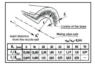
Fig. 10: The negligible effect in Fig. 4 of the transversal curvature is quite surprising, considering the fact that the curvature radius is comparable with the layer thickness  $\delta$ .
