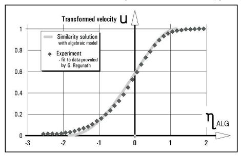
Fig. 18: Comparison of the profiles of relative velocity *u* obtained by the present similarity solution using the algebraic model of turbulence with data points obtained as averages of the values at regular intervals in Fig. 13.
