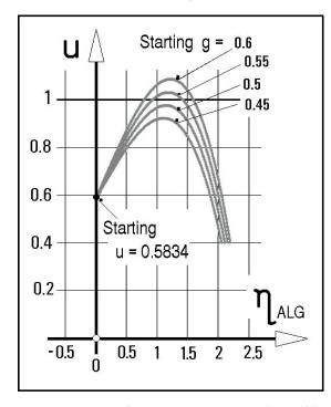
Fig. 15: Solutions for the dimensionless velocity *u* obtained by numerical integration of the set of equations  $df/d\eta = u$ ,  $du/d\eta = g$ , and  $dg/d\eta = -f$  in the direction of the positive transversal similarity co-ordinate  $\eta_{ALG}$ .
