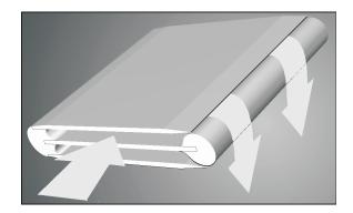
Fig. 6: The principle of supercirculation vanes as successfully developed at CTU in 1973 [9]. The ambichirality required in the present investigations called for two control flow exit slits (and two inlet cavities) in each vane.
