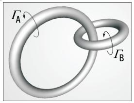
Fig. 3: A high helicity in a fluid flow does not necessarily mean the presence the of helical coherent structures of Fig. 1. Much more important may be the high helicity found for the mutually linked vortex rings (which, according to some theories, may be the basic structures in turbulence).
