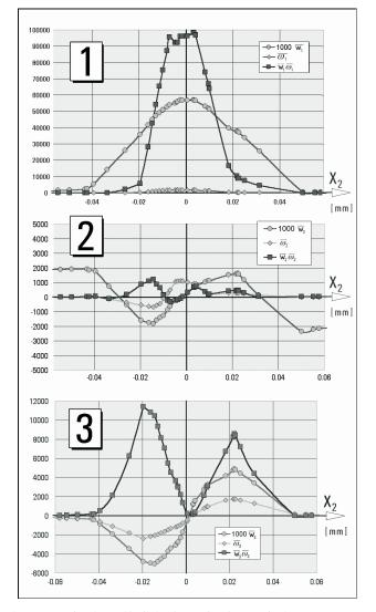
Fig. 19: Evaluation of helicity from the three velocity components and the three components of the vorticity vector. 1– axial components, 2– radial components, 3– tangential components (note the different vertical scales). Computed for 12.6 % relative control flow rate at X<sub>1</sub> = 2 *D*.
