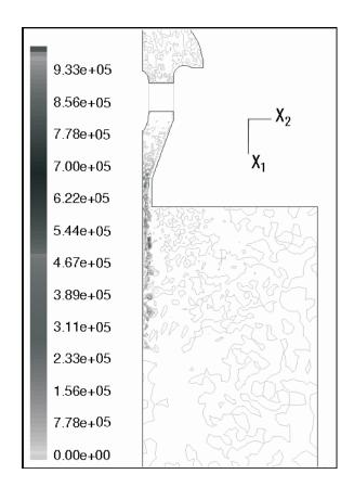
Fig. 15: Typical positive helicity contours evaluated in the meridian plane for a jet with positive swirl chirality – case D, with medium applied relative control flow rate 9.43~%
