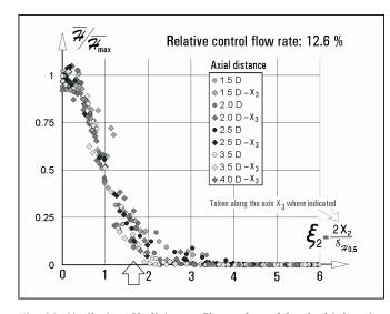
Fig. 23: Similarity of helicity profiles evaluated for the highest investigated control flow rate. The wide arrow (cf. Fig. 17 and Fig. 21) indicates low values, which may be a remnant of the negative wall-layer helicity.
