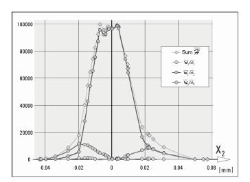
Fig. 20: Profiles of the three velocity × vorticity products from the example in Fig.19 and the helicity profile as the result of their sum
