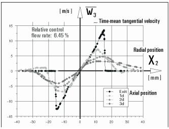
Fig. 13: Typical profiles of tangential velocity and their changes with axial distance downstream from the nozzle exit
