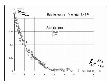
Fig. 22: Similarity the of two helicity profiles from Fig. 21 when plotted in relative co-ordinates
