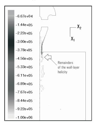
Fig. 16: Negative helicity contours evaluated in the same meridian plane for the same jet with positive swirl chirality as in Fig.15 (the negative valued helicity is generated in the boundary layer on the nozzle wall)
