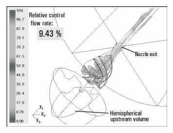
Fig. 11: Computed pathlines (colour coded by velocity magnitude) of the left-hand swirling flow downstream from the swirl generator at a medium magnitude of applied control
