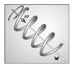
Fig. 1: Helical deformation of a fluid volume in turbulent flows. This idealised shape would arise in the exceptional case of strong rotation with mutually collinear vorticity and velocity vectors.
