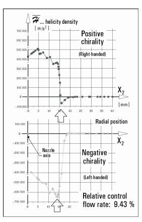
Fig. 17: The consequence of the pseudo-scalar character of helicity: reversal of chirality of the imparted swirl does not lead to a simple change in the sign of the helicity. Halfprofiles of helicity evaluated immediately downstream from the nozzle exit indicate invariance of the sign of the helicity in the nozzle wall boundary layer.
