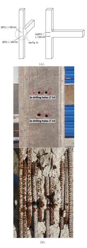
FIGURE 1. Reinforcement of additional bars for model JB0R.
