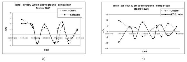
Fig. 1: Air flow 200 cm (a) and 30 cm (b) above ground in two places connected by a tunnel and stairs
