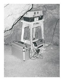
Fig. 3: Radim 3 continual radon monitor in a plastic box with dessiccant, AlphaGuard continual radon monitor, Fritra 4 continual radon and attached and unattached radon daughters fraction monitor for simultaneous measurement of radon concentration and concentration of unattached and attached fraction of its daughters).
