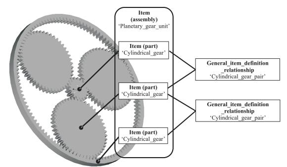
Fig. 6: Planetary gear unit: usage of AP 214 objects with self defined attributes
