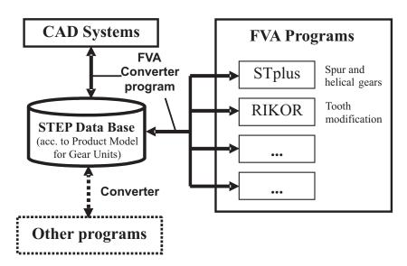
Fig. 8: Applications of the STEP product model for gear units to FVA programs
