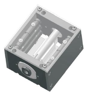
Fig. 2: CAD model of the cold trap module
