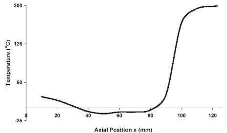
Fig. 3: Absorption/cooling temperature profile within the cold trap module
