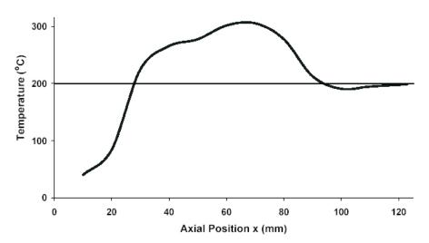
Fig. 4: Desorption/heating temperature profile within the cold trap module
