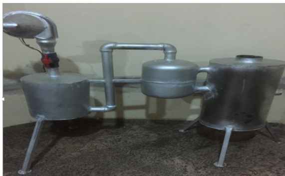
FIGURE 2. The developed downdraft gasifier [37].
