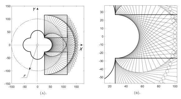
FIGURE 3. Curvilinear profile of four elements, when completely rolling along it, the square makes one turn: a) the set of positions of the square when it is rolling along the arc of the profile; b) enlarged fragment of the profile element
