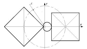
FIGURE 2. Curvilinear profile, with complete rolling during which the square makes quarter of a turn.
