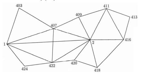
Fig. 2: Example of a local geodetic free network
