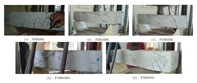
FIGURE 10. Failure mode of RC beam specimens cast with different concrete mixes.
