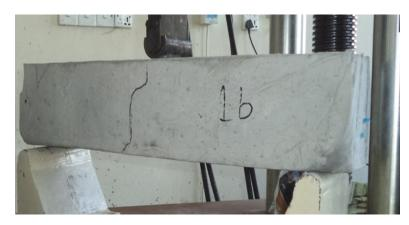
FIGURE 7. Failure mode of sustainable green concrete specimen under bending.
