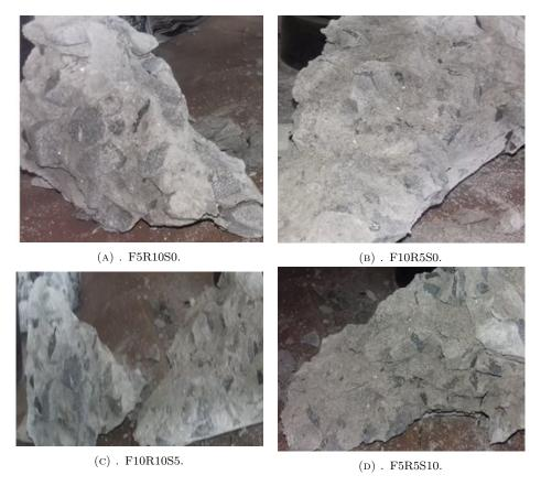
Figure 11. Fracture surfaces of different hardened concrete mixtures.
