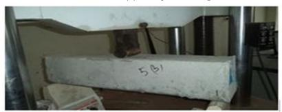
$({\mbox{\bf F}})$  . Flexural strength test.
