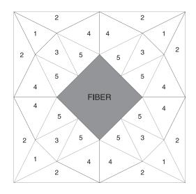
Fig. 10: A simple finite element mesh with groups of elements
