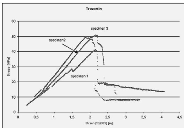
Fig. 9: Stress-strain diagram of a travertine specimen
