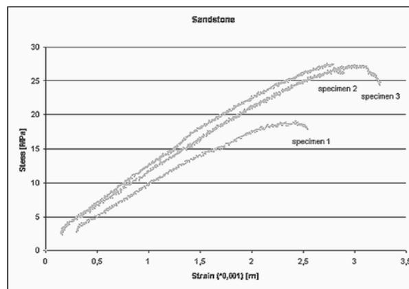
Fig. 4: Stress-strain diagram of a sandstone specimen
