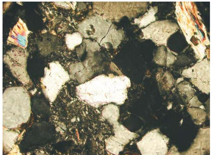
Fig. 1: Micrograph of a thin section of sandstone (in crossed nicols, M = 200)
