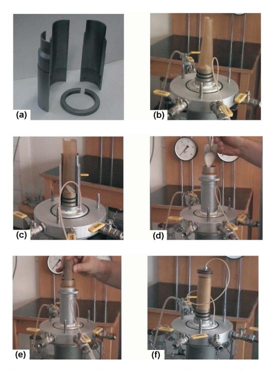
Fig. 2: Steps used for preparing the unsaturated sand samples, (a) the three split mould, and the steel ring; (b) fitting the rubber membrane around the triaxial pedestal and installing the lower O-rings; (c) assembly of the mould around the membrane; (d) filling the mould with sand PR33; (e) compaction of sand inside the mould; (f) sample ready to be tested
