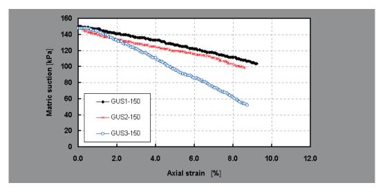
Fig. 6: Variation of matric suction during shearing process of group GUS-150 under constant water content conditions
