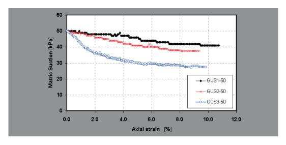
Fig. 5: Variation of matric suction during shearing process of group GUS-50 under constant water content conditions
