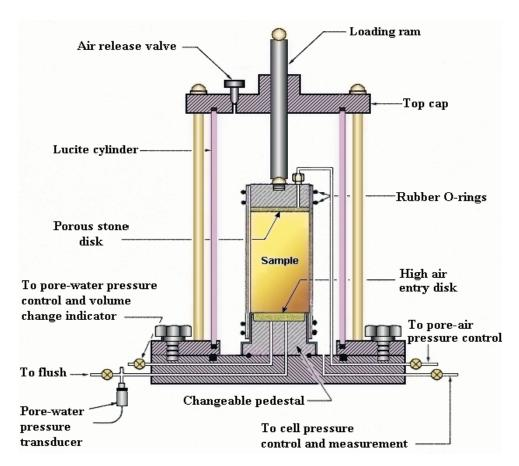
Fig. 1: Longitudinal cross section diagram of the modified triaxial cell for testing unsaturated soils
