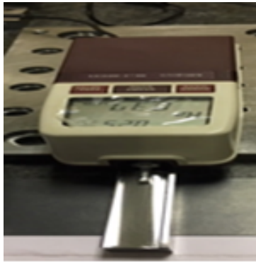
FIGURE 3. Mitutoyo SJ – 201, surface roughness machine.
