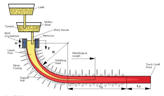
Fig. 1: Main parts of a radial slab caster
