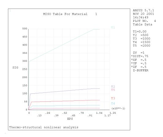
Fig. 3: Stress-strain curves
