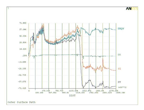
Fig. 4: Stress distribution along the product outer surface
