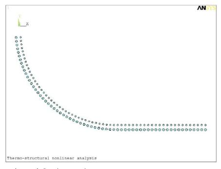
Fig. 2: Roller distribution at the strand of continuous casting
