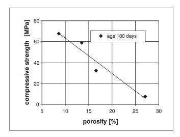
Fig. 4: Dependence of compressive strength on porosity for concrete of age 180 days
