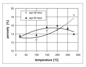
Fig. 7: Effect of temperature on porosity for concrete of age 28 and 90 days
