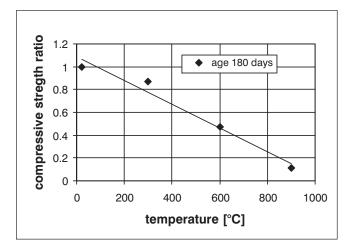
Fig. 2: Effect of temperature on compressive strength ratio for concrete of age 180 days
