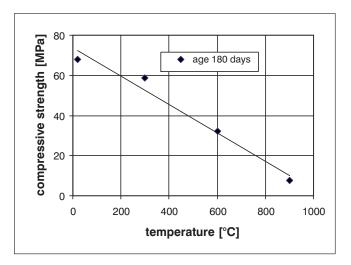
Fig. 1: Effect of temperature on compressive strength for concrete of age 180 days
