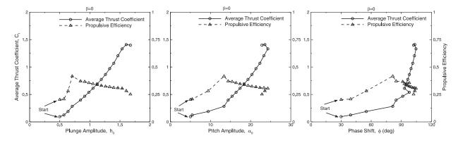
Fig. 5: Maximization of thrust coefficient ( $\beta = 0$ ), Case 1
