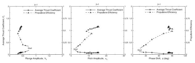
Fig. 7: Maximization of propulsive efficiency ( $\beta = 1.0$ ), Case 3
