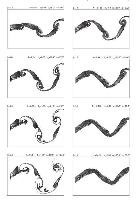
Fig. 8: Instantaneous particle traces at the instant of maximum thrust along the optimization steps for Cases 1 and 2
