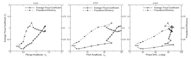
Fig. 6: Maximization of propulsive efficiency and thrust coefficient ( $\beta$  = 0.5), Case 2
