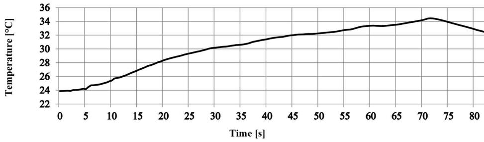
FIGURE 3. Change in temperature vs. time - E100.
