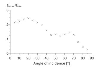
Fig. 2: Dependency of maximum electric field strength inside a housing space referred to incident electric field strength  $(E_{\max}/E_{inc})$  over angle of incidence ( $\alpha$ )
