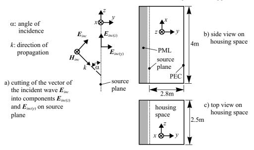
Fig. 1: Simulation of wave propagation and housing space dimensions
