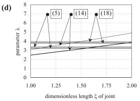
Fig. 5: Parameter  $\lambda$  versus: (a) – transmission ratio u, (b) – width of face  $\psi$ , (c) – operating pitch diameter  $\delta$ , and (d) – length  $\xi$  of the joint. Other parameters are fixed.
