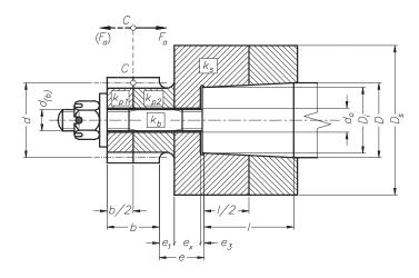
Fig. 3: Definition of spring rates of the considered portions of the frictional joint
