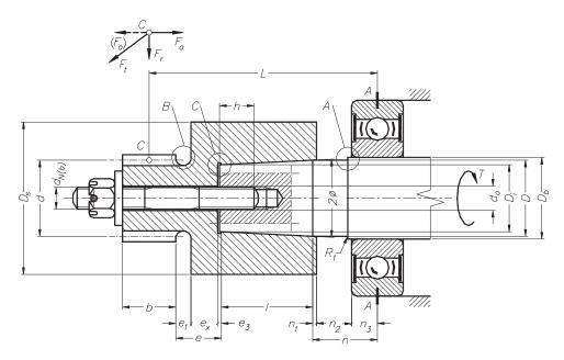
Fig. 1: Geometry of the gear wheel-shaft joint
