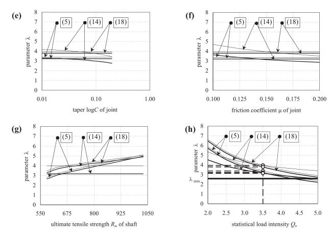
Fig. 6: Parameter  $\lambda$  versus: (e) – taper logC of the joint, (f) – friction coefficient  $\mu$  of the joint, (g) – ultimate tensile strength  $R_m$  of the shaft, and (h) – statistical load intensity  $Q_u$ . Other parameters are fixed.
