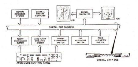
Fig. 2: Typical bus configuration for elementary on board avionics [3]
