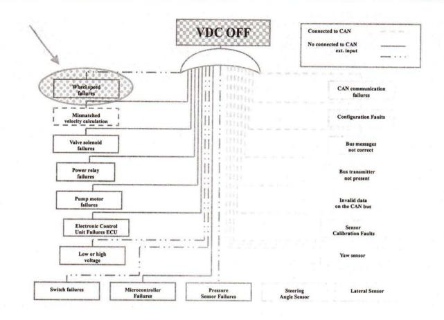
Fig. 5: VDC Fault Tree Analysis
