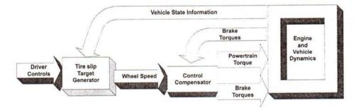
Fig. 7: Traction Control System operational logic
