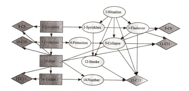
Fig. 3: Bayesian network describing a structure under normal and fire design situations
