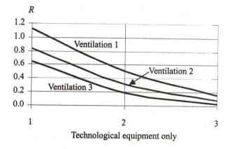
Fig. 6: Effect of ventilation level and technological equipment on expected risk in a tunnel
