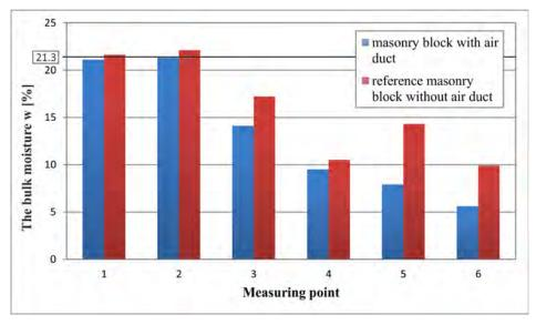
FIGURE 10. The measured values of moisture after 30 days of using the fan.
