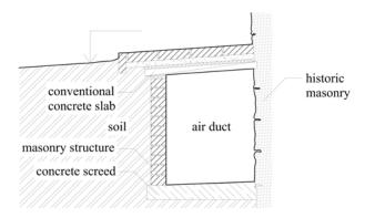
FIGURE 2. The traditional air cavity based on a masonry structure.
