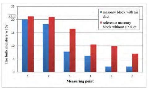
FIGURE 11. The final values of moisture after 90 days of using the fan.
