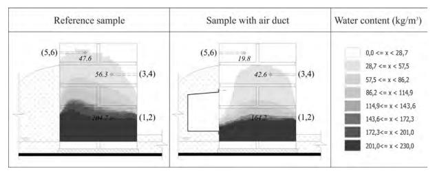
FIGURE 12. The results of the numerical simulation (created in WUFI 2D).
