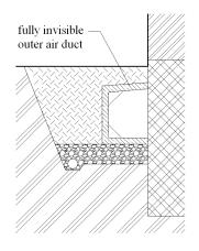
FIGURE 4. Air duct (concrete blocks) installed into a historic masonry building.
