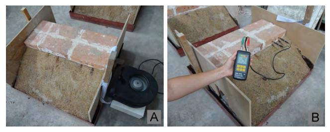
FIGURE 8. (a) Fan providing an air flow in the duct. (b) Measurements made by using of electrical resistivity method.
