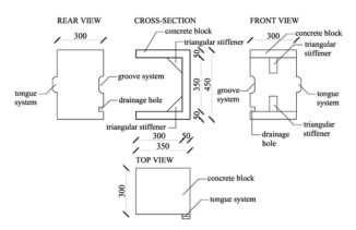
FIGURE 3. A specially shaped concrete block.
