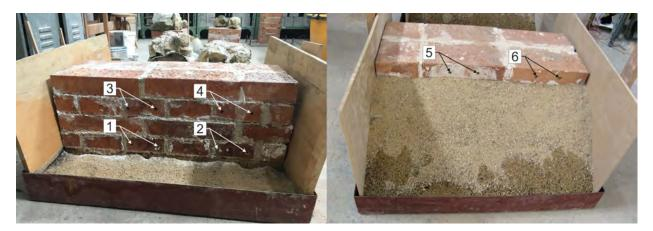
FIGURE 6. Placement of measuring points in masonry (on the laboratory model).
