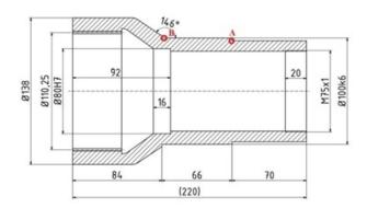
FIGURE 3. Output stage of gear mechanism
