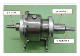
FIGURE 1. Functional model of double-output gear mechanism
