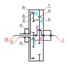
FIGURE 2. Principal scheme of double-output gear mechanism: I – input shaft, II – output shaft, III – output shaft, S – central axis, E – eccentricity,  $z_1$ – $z_6$  – numbers of teeth, 1 – frame, 2 – gear wheel
