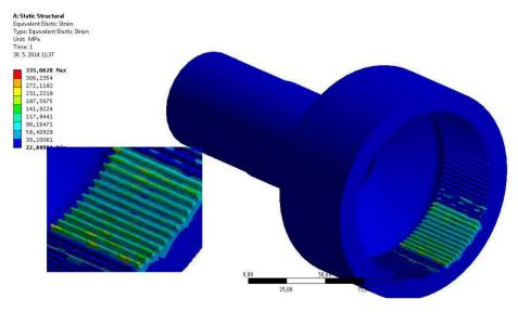
FIGURE 6. Analysis of the gear at the point of contact of teeth.
