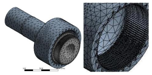
FIGURE 4. Finite element mesh created on the model of the output stage.
