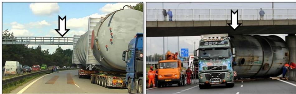
FIGURE 3. Preparing for the underpass of excessive cargo under the toll gate and the situation when the cargo got stuck under the bridge in Ostrava.
