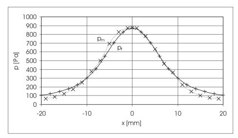
Fig. 4: Dependence of acoustic pressure from K buffer on the x-coordinate at distance z = 6.5 mm,  $f_1 = 20.5$  kHz, generator power 60 %.  $p_t$ - from theory,  $p_m$ - from experiment with microphone.
