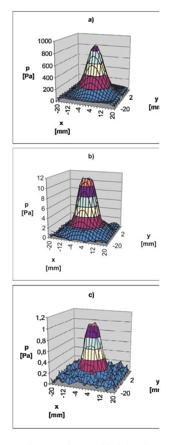
Fig. 3: Microphone measured acoustic field distribution in the *x-y* plane at distance z = 6.5 mm from the buffer K with 60 % power from the generator: a) on base frequency  $f_1 = 20.5$  kHz
