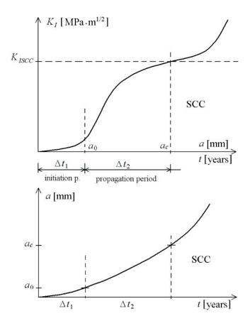
Fig. 3: Fracture toughness vs. time and crack depth
