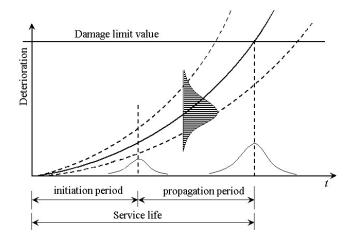
Fig. 2: Two periods of structural service life
