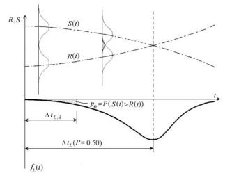
Fig. 1: Probabilistic representation of structural service life
