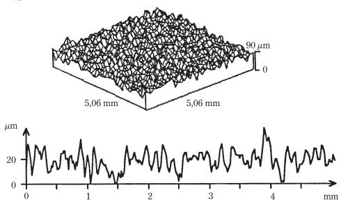
Fig. 1: Representation of surface roughness measurement
