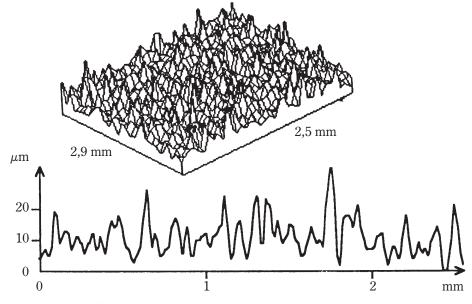
Fig. 2: Representation of surface roughness measurement
