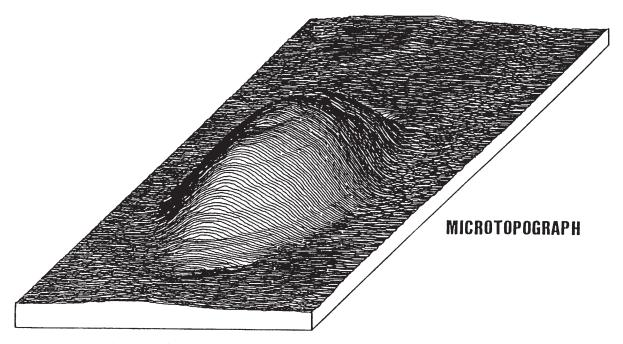
Fig. 6: Microtopograph of a rough surface
